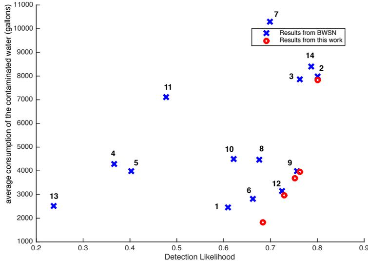
Fig. 2. Detection likelihood and average consumption of the contaminated water with 5 sensors in the 129-Node Network. BWSN labels: 1 = Berry et al.; 2 = Dorini et al.; 3 = Eliades and Polycarpou; 4 = Ghimire and Barkdoll (demand); 5 = Ghimire and Barkdoll (mass); 6 = Guan et al.; 7 = Gueli; 8 = Huang et al.; 9 = Krause et al.; 10 = Ostfeld and Salomons; 11 = Preis and Ostfeld; 12 = Propato and Piller; 13 = Trachtman; 14 = Wu and Walski.
