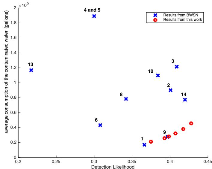
Fig. 5. Detection likelihood and average consumption of the contaminated water with 20 sensors in the 12527-Node Network. BWSN labels: 1 = Berry et al.; 2 = Dorini et al.; 3 = Eliades and Polycarpou; 4 = Ghimire and Barkdoll (demand); 5 = Ghimire and Barkdoll (mass); 6 = Guan et al.; 7 = Gueli; 8 = Huang et al.; 9 = Krause et al.; 10 = Ostfeld and Salomons; 11 = Preis and Ostfeld; 12 = Propato and Piller; 13 = Trachtman; 14 = Wu and Walski.
