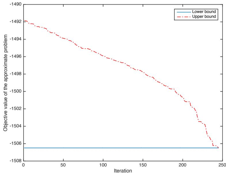
Fig. 6. Progression of the lower and upper bounds with the branch and bound algorithm.
