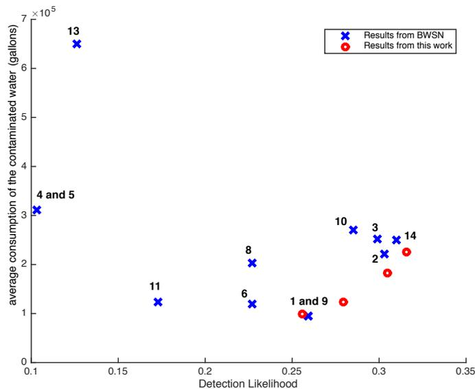
Fig. 4. Detection likelihood and average consumption of the contaminated water with 5 sensors in the 12527-Node Network. BWSN labels: 1 = Berry et al.; 2 = Dorini et al.; 3 = Eliades and Polycarpou; 4 = Ghimire and Barkdoll (demand); 5 = Ghimire and Barkdoll (mass); 6 = Guan et al.; 7 = Gueli; 8 = Huang et al.; 9 = Krause et al.; 10 = Ostfeld and Salomons; 11 = Preis and Ostfeld; 12 = Propato and Piller; 13 = Trachtman; 14 = Wu and Walski.
