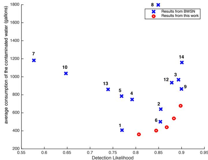
Fig. 3. Detection likelihood and average consumption of the contaminated water with 20 sensors in the 129-Node Network. BWSN labels: 1 = Berry et al.; 2 = Dorini et al.; 3 = Eliades and Polycarpou; 4 = Ghimire and Barkdoll (demand); 5 = Ghimire and Barkdoll (mass); 6 = Guan et al.; 7 = Gueli; 8 = Huang et al.; 9 = Krause et al.; 10 = Ostfeld and Salomons; 11 = Preis and Ostfeld; 12 = Propato and Piller; 13 = Trachtman; 14 = Wu and Walski.
